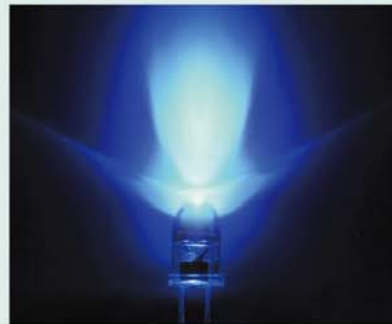
In car headlights, blue LED light incident on yellow or other phosphor generates a bright white light.
