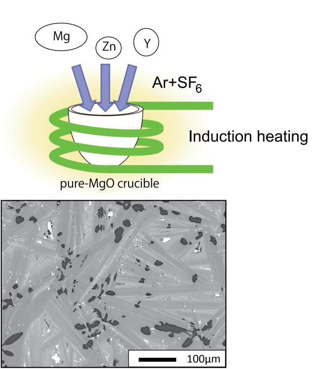
Microstructure of Mg-5at.%Zn-7at%Y alloy
