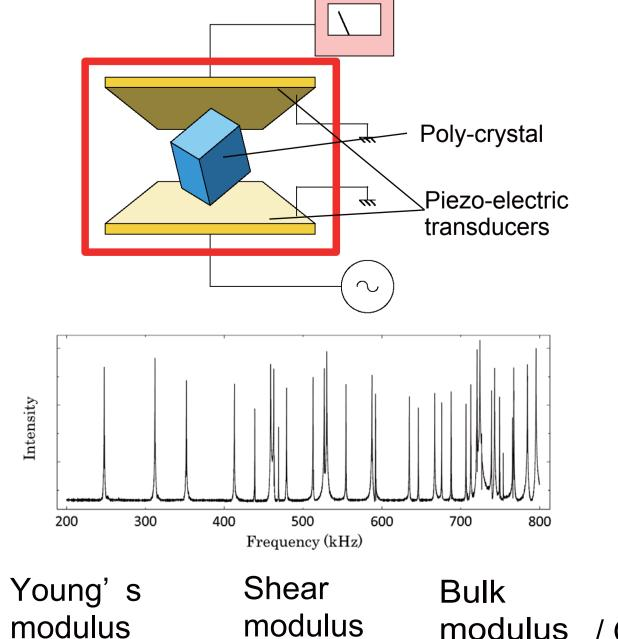
Measurements for LPSO phases with other stacking sequence
