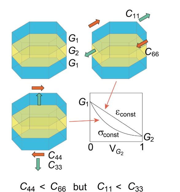
(Resonant Ultrasound Spectroscopy)
