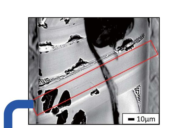
A small single crystal was cut out (20 X 30 X 100 µm<sup>3</sup>)
