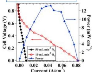
The shape of the polarization plots of the MEA cell was similar to that of a standard fuel cell, demonstrating that the system can stably produce electricity by H<sub>2</sub> and O<sub>2</sub> gases.
