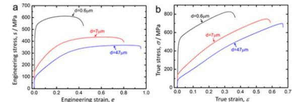
Mechanical properties of Cu-15Al specimens with different grain sizes
