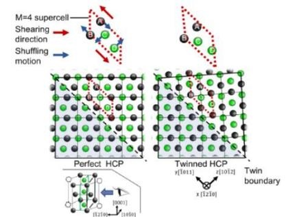
Atomic arrangements and four-atom supercell shape of perfect HCP and twinned HCP configurations
