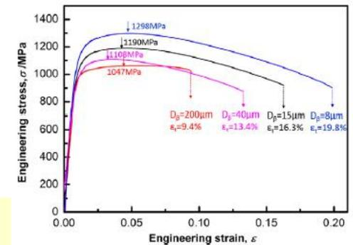
Engineering stress-strain curves of fully martensite microstructures with different  $\beta$  grain sizes
